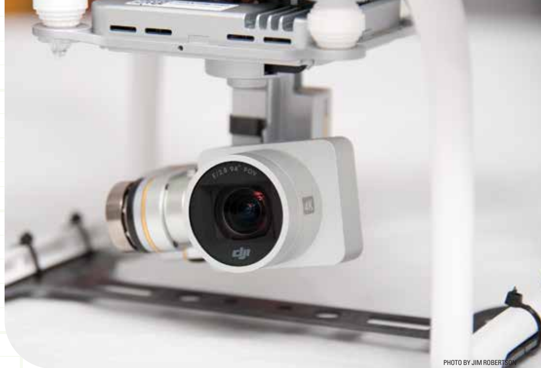
▲ The DJI Phantom drone model Somerset Police are using has its own, integrated camera. When choosing a drone for your agency, knowing which ones have an integrated camera and which ones allow you to mount your own is important. The quality of photos and video produced by an integrated camera also should be considered.
